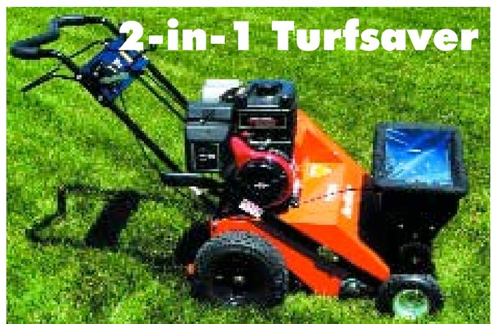
TURFSAVER, from DJ Turfcare, is a new machine from the US that de-thatches and overseeds (or fertilises) in one compact unit. It's ideal for contractors, greenkeepers and groundsman, it comes fitted with blades to verti-cut and covers a 22-inch wide swathe in a single pass. Turfsaver is manufactured by SourceOne, designers of the Plugger aerator.
